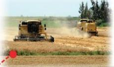
Crop yield maps are created while reaper and combine harvesters are working on the field. Meanwhile remote sensing models are calibrated with the acquired yield data. In this way farmers can track the expected yield of their crops as from the sowing phase.
