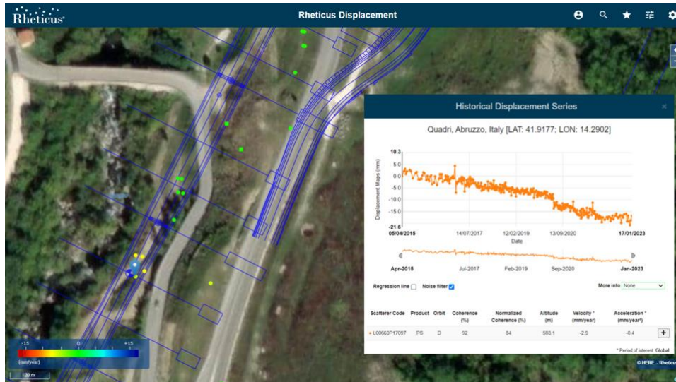
Fig. 4. Ground motion service provides regularly updated nation-wide maps of millimetric ground movement based on data from Copernicus Sentinel-1 mission
